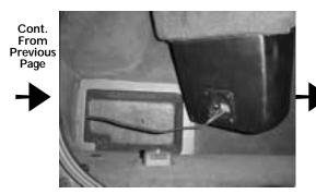
**STEP 7: (a)**Run speaker wire form the amplifier's location to the Stealthbox's® terminal and connect.
